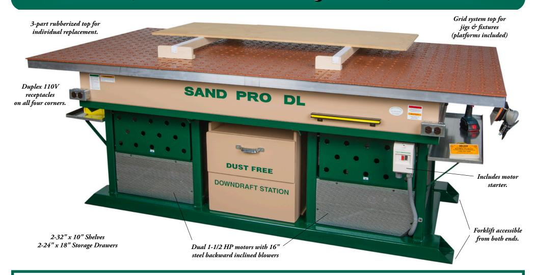
The DL9648 is a dedicated 8' by 4' sanding table that doubles as a workbench. It features 4-duplex receps, a grid system top, two 10"x 32" shelves, two 18" x 24" storage drawers, has easy filtering service, is forklift accessible from both ends, and uses two TEFC 1-1/2 HP motors. The SAND PRO DL9648 is perfect for sanding large pieces such as house doors or as a multi-person sanding station.
