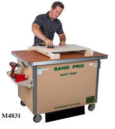
K-There is no need to rob valuable C.F.M. from your central vacuum" system or conditioned air from your shop. Machine remains truly" portable with no interference from a long vacuum hose.
